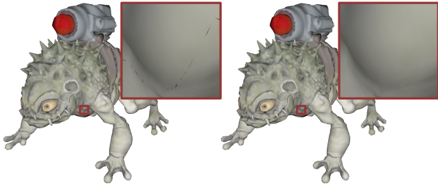
Figure 9: Example for multi-signal: the left image shows the original Monster Frog model displaced and colored by textures, the right image shows our rendering, where displacement, normal, and color were stored as tessellator attributes. The left close-up shows the cracks that are common along chart boundaries when using displacement textures. Our representation (right) does not suffer from such artifacts.
